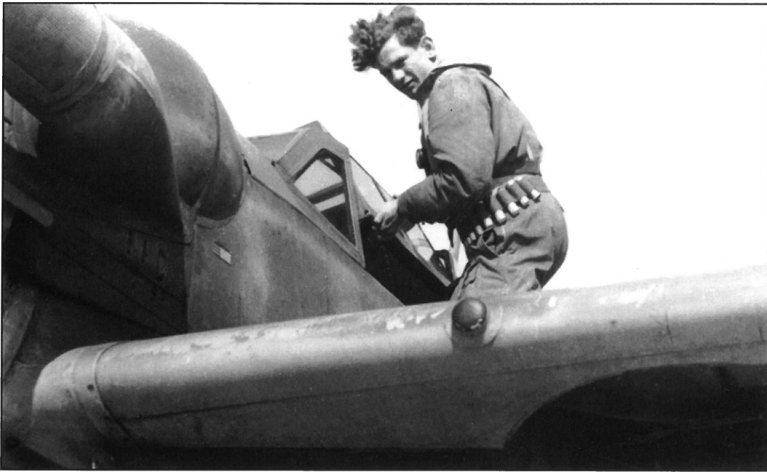
The tropical filter and lack of umbrella holders can be seen. Note the factory data plate. The gun camera aperture on the port wing is capped over.
