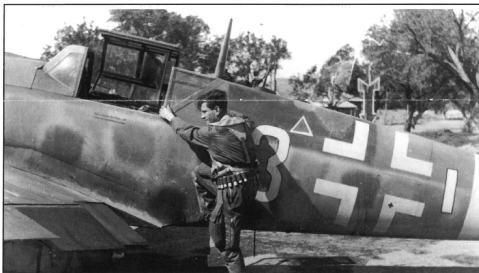
Close-up showing this unusual large spots of RLM 74/RLM 75 and the fuselage. The slightly larger than standard (900 mm) White outline fuselage cross is interesting.
