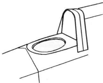
Assembly of main cockpit component inside the left fuselage side
