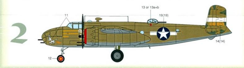
"The Gay Mare," a B-25D-1 of the 501st BS, wears standard Olive Drab/Neutral Gray warpaint, Medium Green mottling, red cowl rings, white fin & rudder I.D. bands (inside and outside surfaces) and overpainted nose glazing. Note the colorful nose wheel hub device. It crashed in bad weather 30 Aug. 1944.Pilot at the time of this profile was 1" LT. Lawrence Schrade.
