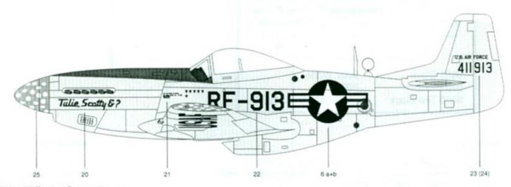
RF-51D, 44-11913, 45th Tactical Reconnaissance Squadron, 67th TRG, Kimpo AB, South Korea, 1951. Overall natural metal with medium blue (approx. F.S. 15102) spinner, wingtips and tail tips. Anti-glare panel Olive Drab. Tip of vertical tail is yellow. Note camera ports in rear fuselage and DF loop on spine.
