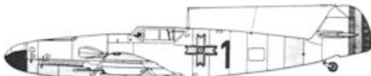
BF-109G-6 2/R-8, White 1, 1st Air Corps, Rumanian Air Force, 1943. Flown by Rumanian Ace, Capt. Alexandru Serbanescu. Standard 74/75/76 scheme with G2/70/74 mottle. Tail band, lower cowl and lower wingtips yellow. Segmented spinner in RLM 70 and white. Note underlying cannon gondolas.
