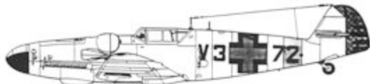
BF-109G-6 (late production), W472, Royal Rumanian Air Force, 1944. Standard German 74/75/76 camouflage with G2/70/74 fuselage mottle. Spinner is 1/3 white and 2/3 RLM 70. Markings in yellow. White theatre band on aft fuselage and lower wingtips. Note late D-6 type antenna mast and cockpit canopy stowage attachment points.
