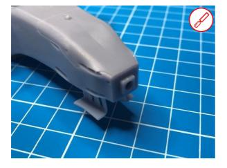
At the rear edge of the wing elements of the front wing is a sensor on both sides. The support structure still has to be removed here.
