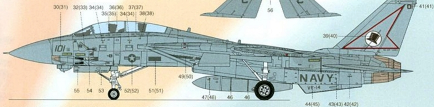
F-14A BuNo. 162691, 'Camelot 101' of VF-14 "Tophatters", USS John F. Kennedy, Operation Desert Storm, Jan/Feb 1991. Upper surfaces Dark Ghost Gray, lower surfaces Light Ghost Gray. The finish of this aircraft was extremely weathered and mottled with paint touch-ups, and major warnings repainted in nonstandard fashion in Gunship Gray (FS 36118). Most standard small stencilling was oversprayed and not redone.
