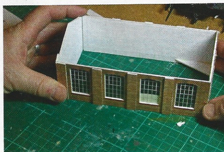
12 Glue the two wall sections together, ensuring that the joints are level and square in all directions. Allow the glue to become tacky, and hold them in place for a couple of minutes while the grip takes effect.
