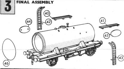
20. Cement tank barrel to underframe locations.
