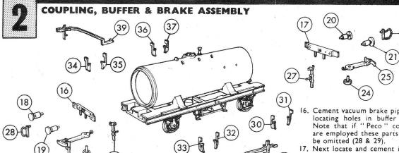
10. Locate and cement buffer beams to ends of underframe (16 & 17).
