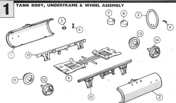
It is recommended that the instructions and exploded view are studied and that the assembly is practised before cementing together.
