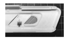
Step two.Drill a series of holes at the part, with a 1.5 mm drill bit.
