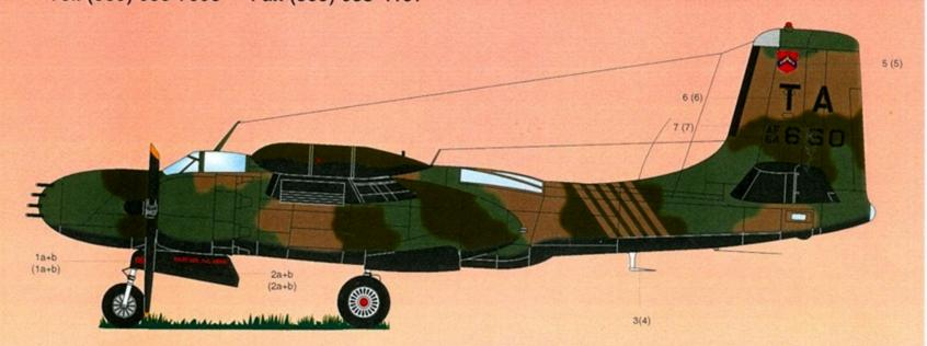
AIRCRAFT 1 • Douglas (On Mark) B-26K 64-17660, 609th Special Operations Squadron, Nakhon Phanom, 1969. Aircraft flown by Squadron Commander, Colonel E. J. White. Standard SEA Green 34102/Green 34097/Tan 30219 uppersurfaces with Black undersides. Note gray fin tip, black propeller spinners and red hubs on all wheels. No national insignias were carried on this aircraft.
