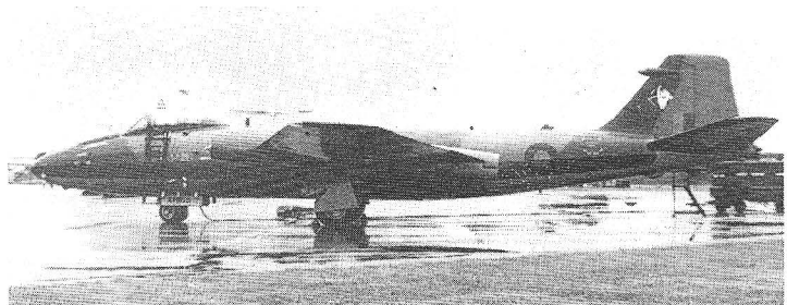
1. Canberra PR.9, XH165 of No. 1 P.R.U., Wyton, seen in mid-1985 at RAF Brize Norton; its gloss finish is not due to the obvious weather conditions — unlike the other Canberra variants still in service at Wyton, the PR.9s are in high gloss finish. Note the crew ladder in place, and the prominent PWR 'bullets' on the fin and rear end of the fuselage. Photo: J. Kyte
