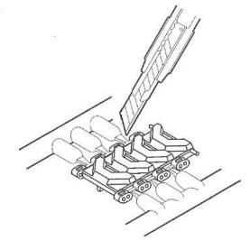
\* 履帶安裝完整一側需要標准77節 Complete track for one side requires 77 links
