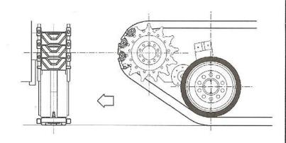
\* 配備主動輪、誘導輪。 Resin Made Drive Sprocket and Idler included.
