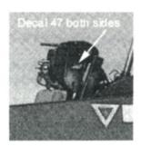
Decals no. 47 are to be applied either side of the ejection seat
