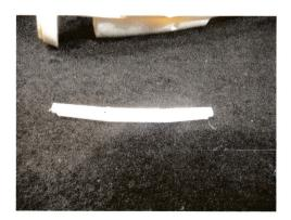
Carefully sand the backing excess from the forward nose piece and glue into place on the assembled fuselage. I recommend thick Gorilla glue. The top of this piece has a notch in it.
