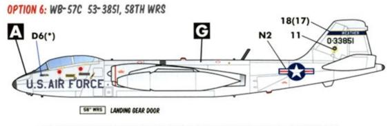
WHILE THE WB-57C'S OF THIS UNIT WERE EQUIPPED WITH A SAMPLING POD AS SHOWN, THEY WERE ALSO SEEN WITH STANDARD TIP TANKS.
