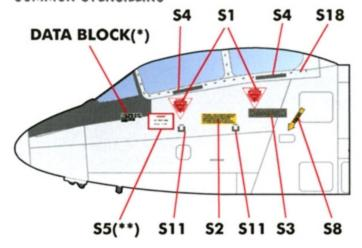
MARKINGS ON THE CANOPY FRAME (\$18 AND \$4) ARE SHOWN IN BLACK FOR CLARITY. CUT AND APPLY \$18 ON THE CANOPY FRAME AS SHOWN.
