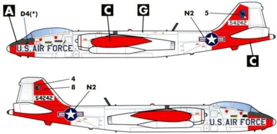
ALL EB-57 OPTIONS ON THIS SHEET ARE EQUIPPED WITH THE AN/ALE-2 COUNTERMEASURES POD UNDER THE WINGS. THIS POD IS NOT PROVIDED IN THE AIRFIX KIT. LONE STAR MODELS OFFERS A RESIN VERSION.
