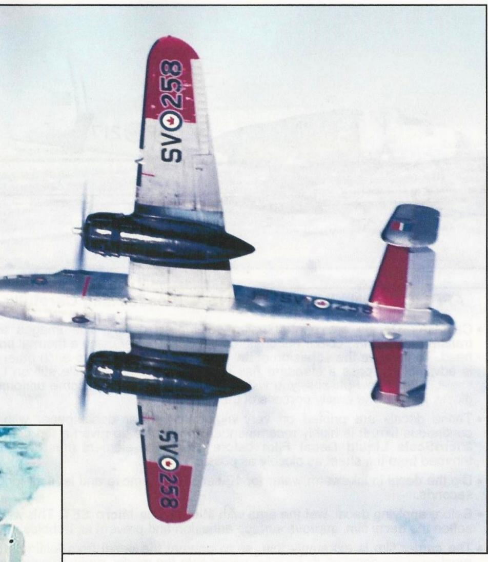
system where the top S-shaped stacks were replaced by semi-collector rings.
