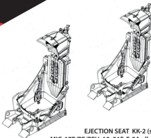
EJECTION SEAT KK-2 (suitable for MIG-17P/PF/PFU, 19, 21F, E-2A all model kits)
