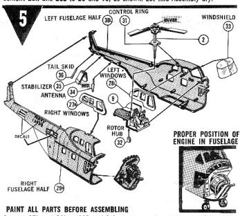
Cement 27R and 28L to 29R and 30L, as shown. Carefully cement STEP 3 to inside of 30L. Slide 31 onto 2, and slide 2 down through Hole in Part 9, as shown. 2 locates into Large Slot and 31 locates into Small Slot in Fuselage, as shown. Cement 32 to 2 underneath 9, as shown. Now cement 29R and 30L together, locating STEPS 2 and 3 properly. Cement STEP 4 in place, pushing Assembly until it rests against Stops. Cement 33, 34, 35 and 36 info place. APPLY DECALS AND SET ASIDE TO DRY
