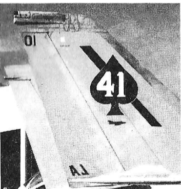
Left and right vertical stabilizers on 160403. Note that one hoist marking is missing on the right stabilizer, and although originally painted, the leading edges show wear. Carefully note the style of the AJ. (VF-41)
