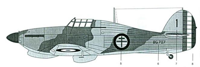
Hurricane Ilb, BG707, Free French forces attached to the RAF, North Africa, 1942. RAF Dark Green, Dark Earth and Azure Blue camouflage. Large area of fuselage and vertical tail overpainted with Mid Stone. Spinner black. 49" Type B roundels on upper wing and 50" Type A on lower wing available on AeroMaster Sheet 48-026.
