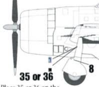
Place 35 or 36 on the front side of the landing gear strut assembly.
