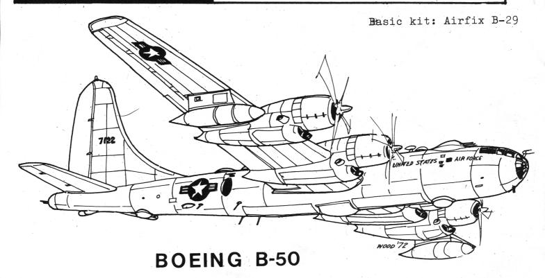
Originally called the XB-44, the B-50 was to have been a converted B-29 Superfortress with R-4360 engines to replace the R-3450s of the B-29. While externally similar to the B-29, the B-50 was in fact an 80% re-design. The B-50 was not only used as strictly a bomber aircraft but was also used as a reconnaissance aircraft, crew trainer, tanker and ultimately weather reconnaissance aircraft.
