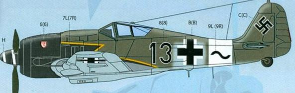
FW 190 A8/R8 of JG3. A/C appears to be camouflaged in RLM 74/ 75/76, although the whole fuselage is in RLM 74, with a light patch of RLM 76 behind the cross. Upper deck guns were remove to compensate for the extra weight of steel armor plating on the fuselage and the armored glass panels.
