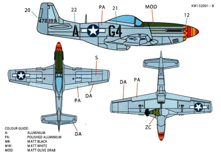
NOTES: The wing surfaces of the P51D were filled and smoothed, removing all surface detail except for fine gaps between panels. This surface was then painted silver - not left as bare metal as is easily assumed from its appearance in photographs. Very little if any rivet detail was visible after this process. This ensured smooth, uninterrupted airflow over the laminar flow wing. All other surfaces (except where indicated) were left bare metal.
