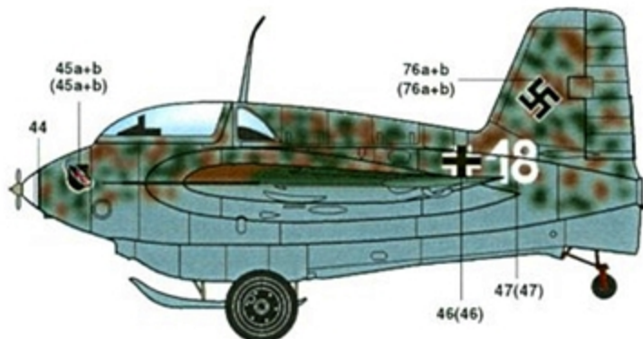
The Me163B-0 flown by 2./JG400's Jupp Mühlstroh wears a fuselage finish of mottled RLM81 and RLM82 over RLM76. Note the White nose tip with thin Black edging (decal 44). Generator prop is worn aluminum.
