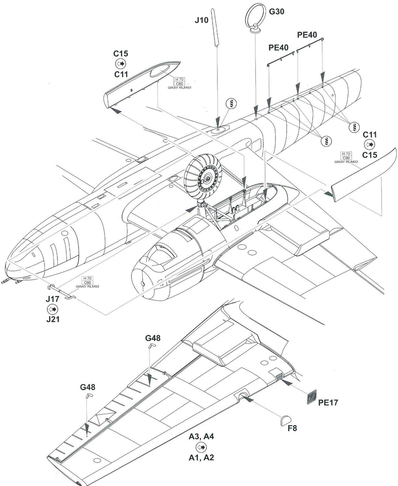
**WE RECOMMEND TO GLUE J24/J32 EXHAUST BASES TO ENGINE NACELLES FIRST, NEXT GLUE THE EXHAUST PIPES TO THE BASES.**
