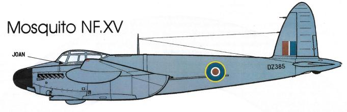
Mosquito NF,XV, DZ 385, of af 85 Sqn in 1943. The aircraft is finished in overall PRU Blue. Spinners and radome are Night. Small White K is located on the front lower portion of the nose radome.
