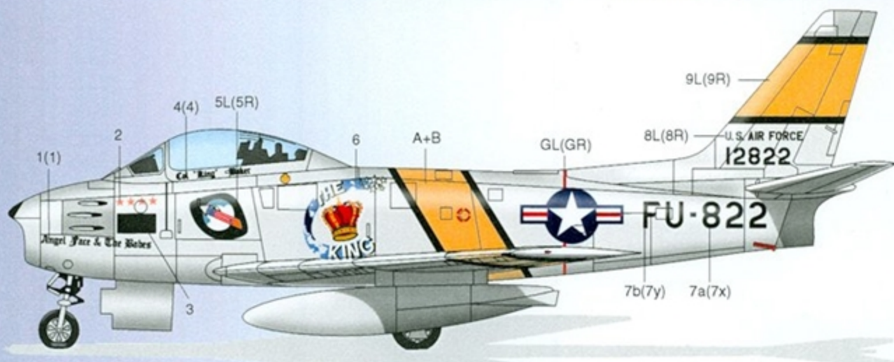
"ANGEL FACE & THE BABES" Colonel Royal N. Baker Commander, 4th. Fighter Interceptor Wing, F-86E-10 #52- 2822. 336th. Fighter Interceptor Squadron, Kimpo 1952. Slatted wing.
