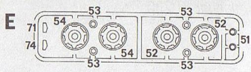
Remove chrome paint where parts are to be glued together
