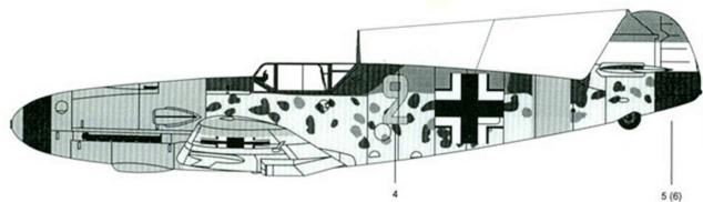
Bf-109F-4, 1/1 Vadasz Század, Hungarian Air Force, Stalingrad, 1942. RLM 74/75/76 camouflage with yellow spinner tip, cowling, lower wing tips and fuselage band. Rear of spinner RLM 70, possibly with 1/3 white.
