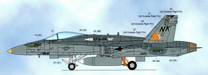
AIRCRAFT 2 • F/A-18C, BuNo. 163719, #200 flown by CAG Captain Tallent, VFA-115 'Eagles', NAS Lemoore. Note "Yellow Socks" coloring of main undercarriage struts. In addition to stencils 22,23 and 24 provided, aircraft apparently had minimal standard stencilling.
