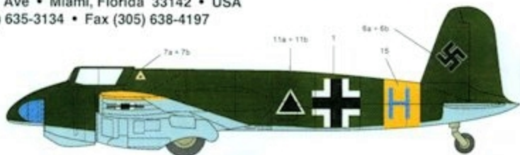
Hs 129B-1/R2, 4(Pz)/Sch.G.2, Russian Front, August 1943. RLM 71 Dunkelgrün upper surfaces with RLM 65 Hellblau beneath. RLM 24 Blue spinner with RLM 04 wing tips and fuselage band. Note that the fuselage band is slightly wider than normal.
