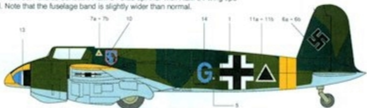
Hs 129B-1/R22, 4.Sch. Gr. 1, Russian Front, Summer 1942. Standard "splinter camouflage" scheme of RLM 70 Schwarzgrün and RLM 71 Dunkelgrün upper surfaces and RLM 65 Hellblau under surfaces. Spinner is RLM 70 Schwarzgrün or black with a RLM 24 Blue Tip. Nose, wing tips and fuselage band are RLM 04 Gelb.
