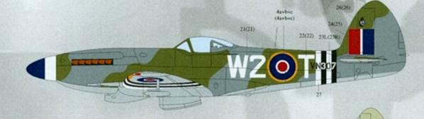
VP459 Scrap view showing pre-July markings and camouflage as an alternative scheme.
