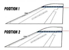
THE TAIL BAND WAS PLACED IN TWO DIFFERENT POSITIONS AT DIFFERENT TIMES. THIS REQUIRES BANDS OF DIFFERENT LENGTHS.
