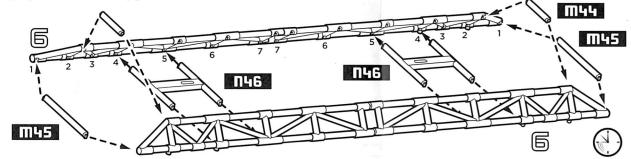
Dry fit each part in place then apply liquid cement to the joint allowing capillary action to bond parts. Install all parts M44 before beginning to install parts M45.
