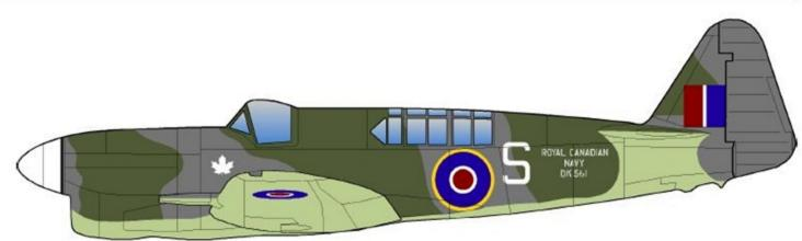
sides, 50" Type B roundels above the wings, 32" Type C below. Royal Canadian Navy and serial number were in stencilled 4" white lettering. Spinner was white. The aircraft code letter was white as was the maple leaf on the forward port fuselage.
