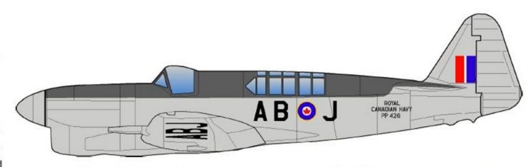
a yellow ring) on the fuselage sides and upper wings. Below the starboard wing, VG in 36" black letters; under the port wing ABJ. Royal Canadian Navy and serial number in 4" black stencilled letters.
