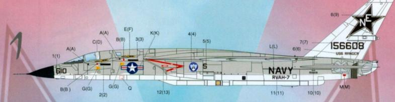
RA-5C Vigilante BuNo. 156608. The *Peacemakers* of RVAH-7 were aboard USS *Ranger* (CV61) for the squadron's final cruise, to WestPac in 1979. Non-specular Gull Gray FS36440 upper surfaces with Gloss White FS17875 vertical fin, undersides, control surfaces, landing gear, wheel wells, and fin tip antenna. Wing leading edge slats Dark Gull Gray FS35231; radome was Flat Black FS37038 and the edges of gear doors were painted FS11136 Insignia Red. Black radome.
