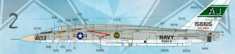
RA-5C Vigilante BuNo. 156615. Vigi operated by the *Hoot Owls* of RVAH-9 aboard USS *Nimitz* (CVN68) for her 1976/1977 Med cruise. Non-specular Gull Gray FS36440 upper surfaces with Gloss White FS17875 vertical tail, undersides, control surfaces, landing gear, and wheel wells. Wing leading edge slats Dark Gull Gray FS35231; edges of gear doors FS11136 Insignia Red; radome was faded tan, approximately FS23717.
