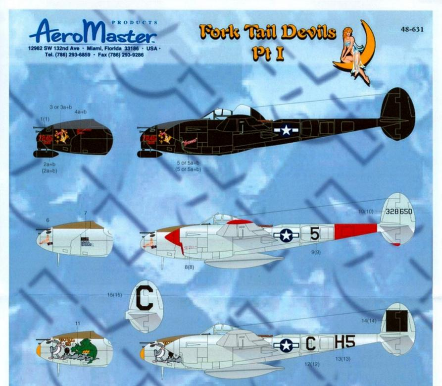
P-38M, 418 NFS, flown by 1st Lts. Johnny Brewer and David Hopwood during the occupation of Japan, late1945. Gloss Black with Flat Black A/G panel. N.M. turbocharger exhaust areas. This A/C was heavily stained on top of booms and across fins and rudders. Note Flame Damper shrouds at the end of the armament. The name Snooks may have been on both sides.
