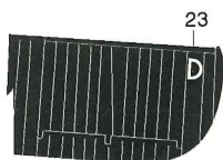
LS231 White aircraft code 'D' is situated approximately between 2nd & 3rd ribs on under surface of mainplane. Both port & starboard codes face same way.
