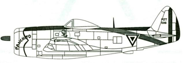
All aircraft depicted are P-47D-35s and higher which require the addition of a dorsal fin. These aircraft were all fitted with a paddle bladed Curtis Electric propeller. Sources for this prop are Monogram's B-26 Marauder and P-47D Razorback kits (with modifications).
