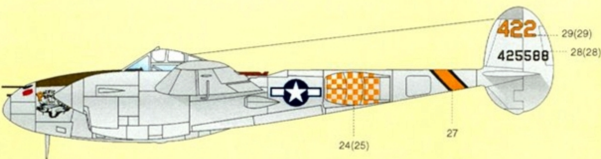
P-38L-5-LO, 44-25588, "Pacific Prowler", 44th Fighter Squadron, 18th Fighter Group, Moret Field, Zamboanga, Mindanao, Philippines, 1945. Flown by 2Lt. Clint Ward. Overall natural metal finish with standard olive drab anti-glare panels. Note left hand .50 cal. machine gun removed and opening covered over and painted red (decal no. 1). Open spoked wheels had natural metal hubs.
