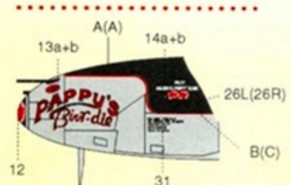
P-38L, "Pappy's Brr-die", 431st FS, 1945. Flown by Maj. R.I. "Pappy" Cline. Overall natural metal. Black anti-glare panels on nose & inboard side of engine nacelles with red trim on nose panel. Rear section of spinners red. Upper & lower tips of tails red with thin black stripes.
