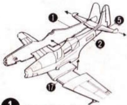
**1** Assemble the fuselage and the wings.
