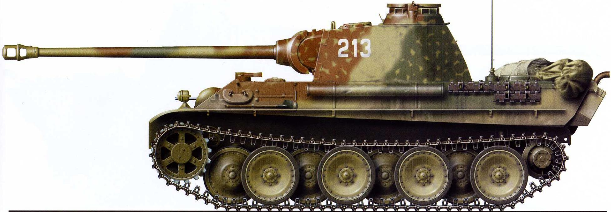
Pz.Kpfw. V Panther Ausf. G, coded "213", of 31st Panzer Regiment, 5th Panzer Division; Goldap area (Poland), November 1944. The tank was delivered to the unit in the autumn. Of note is the lack of Zimmerit and interesting camouflage pattern, which consists of brown and green spots of different size with some dark yellow accents.
