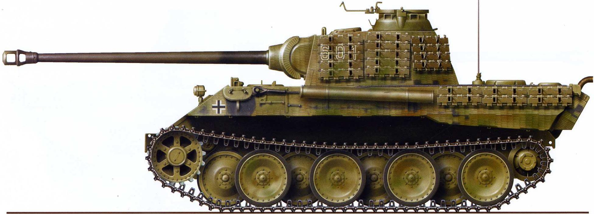
Pz.Kpfw. V Panther Ausf. A, coded "601", of 23rd Panzer Regiment, 23rd Panzer Division; Poland, August 1944. The tank has numerous spare track links attached to the turret. Tactical number, painted on the spare tracks in white outline only, is barely visible.
