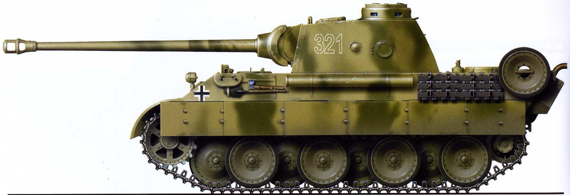
Pz.Kpfw. V Panther Ausf. D, coded "321", of 2nd SS Panzer Regiment, 2nd SS Panzer Division; Russia, summer 1943. The battalion arrived at the eastern front with merely 71 tanks on strength. They were finished in dark yellow color, with splotches of olive green. Spare road wheels mounted to the rear of tanks' hulls were a distinctive feature of the vehicles from this unit.
