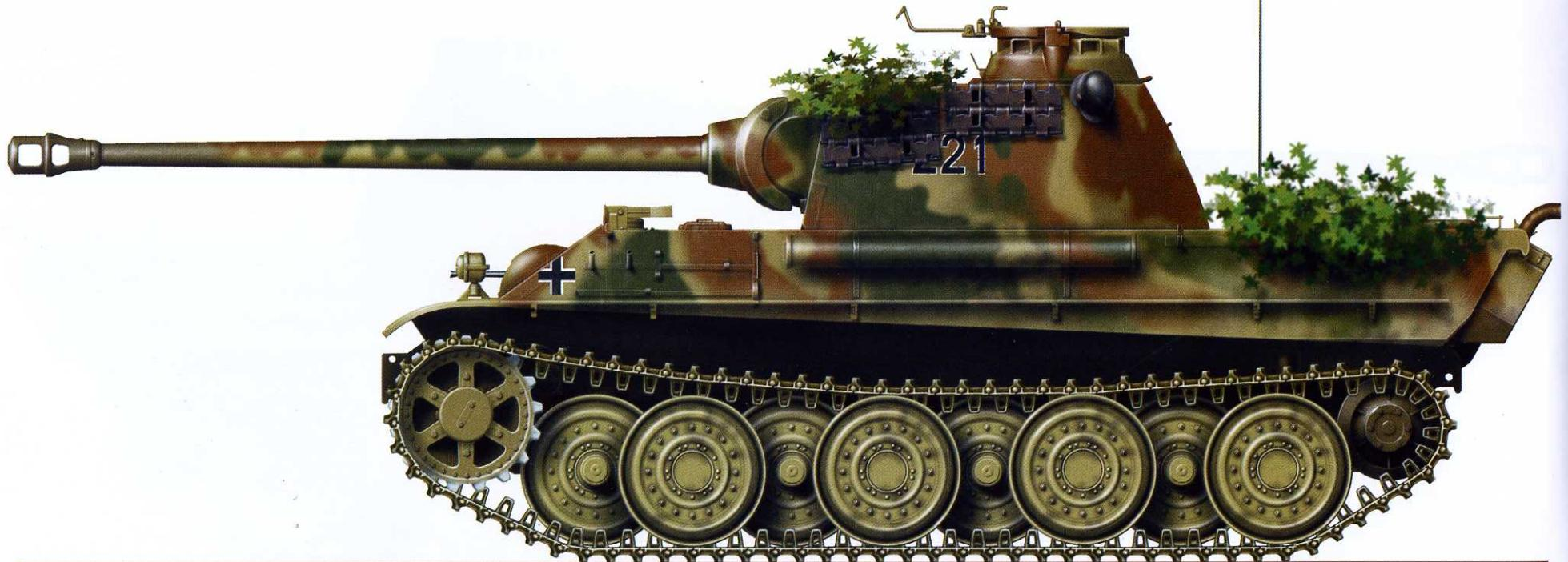
Pz.Kpfw. V Panther Ausf. G, coded "221", of SS-Scharführer Knappich, 1st SS Panzer Regiment, 1st SS Panzer Division; the Ardennes, December 1944. The tank is fitted with steel-rimmed road wheels. This Panther was lost in late December 1944 at La Gleize. Spare track links attached to the turret partially obscure tactical number.
