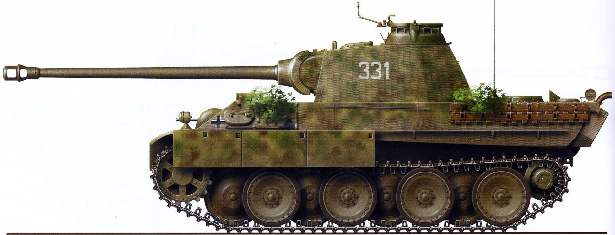
Pz.Kpfw. V Panther Ausf. G, coded "331", of Lt. Goldhammer's company, 35th Panzer Regiment, 4th Panzer Division; Poland, July 1944. A distinctive feature of Panthers from this unit was that the container for spare antennas and bore brush was moved from the side to the rear deck, just above exhaust pipes. The tank's camouflage comprises three-color, irregular dappling.
