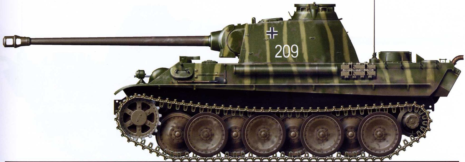
Pz.Kpfw. V Panther Ausf. G, coded "209", of Panzer Division 'Feldherrnhalle 2'; Czechoslovakia, spring 1945. This is a vehicle of final production series. Due to shortage of dark yellow paint, olive green was used in this case as the base color.
