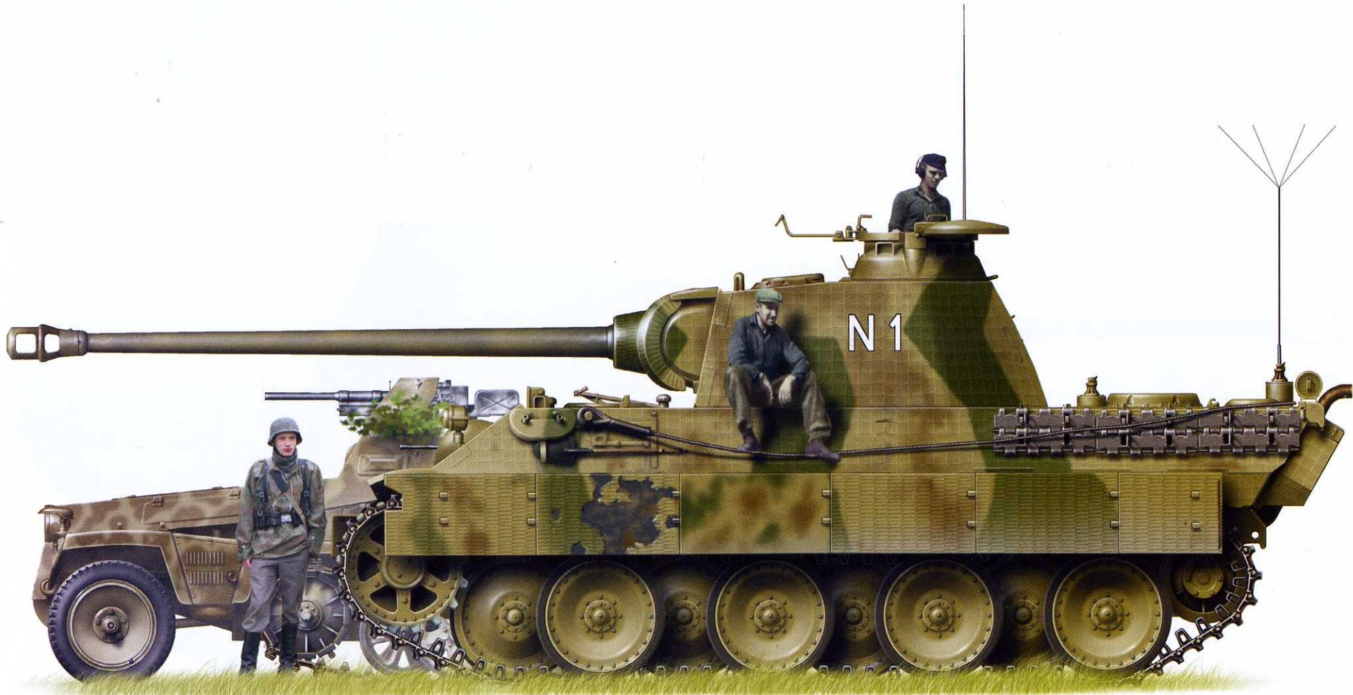
Pz.Kpfw. V Panther Ausf. A, coded "N1", of Maj. Pössl's I Battalion, 'Großdeutschland' Panzer Regiment, Panzergrenadier Division 'Großdeutschland'; Latvia, summer 1944. This is a command vehicle. Like most vehicles of this unit, the tank has the container with bore brush and spare antennas moved to the rear deck.
