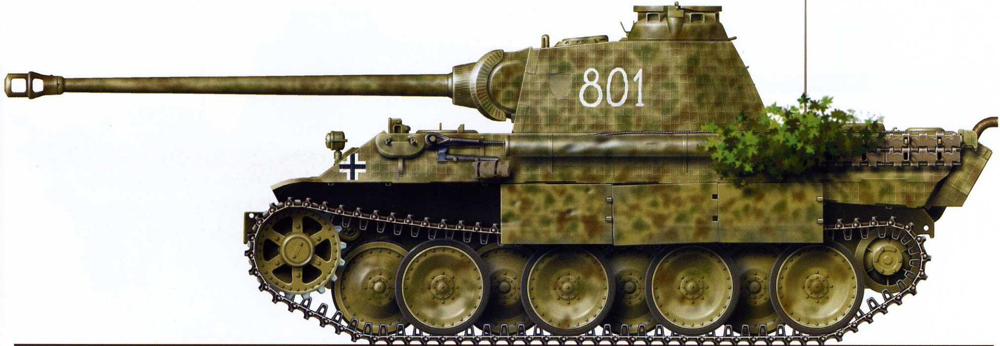
Pz.Kpfw. V Panther Ausf. A, coded "801", was the mount of the CO of the 8th company, SS-Untersturmführer Nicolussi-Leck, of 5th SS Panzer Regiment, 5th SS Panzer Division; Poland, August 1944. The tank carries a hand-painted tactical number. Of note is a shield-shaped patch of removed Zimmerit ahead of the code, apparently to make room for the unit's badge. However, badges were not painted in this spot.
