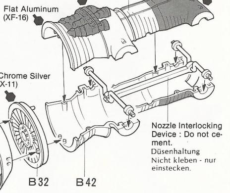
Nozzle Interlocking Device : Do not cement.
