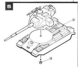
NOTE: Do not cement turret to hull. Insert turret swivel pin into hole in hull and cement retainer ring to swivel pin only.
