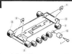
Place metal axles in hull bottom. Cement the four (4) axle retainers against the inside of walls of hull.
