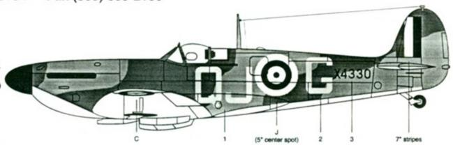
Spitfire Mk.I, R6595 (serial overpainted), 610 County of Chester Sqdn, RAF Biggin Hill, August 1940. Dark Earth, Dark Green & Sky camouflage (Type B pattern) with black spinner. Fin flashes (5° stripe widths) incorrectly applied with blue portion facing foward, this aircraft only. No lower wing roundels.
