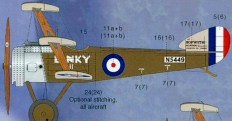
Aircraft 3 - Sopwith Triplane, 8 Naval Squadron, St.-Eloi, France, May 1917. PC10 Camouflage consists of Khaki uppersurfaces and clear doped undersurfaces. NMF cowl. This a/c was used by aces Johnston, Crundall and Spence. Notice doped linen vertical fin with full Sopwith titling on it.
