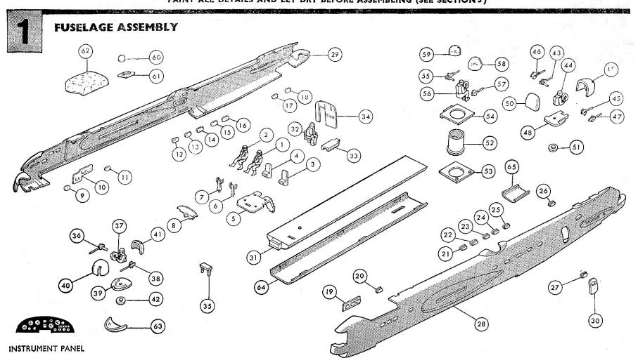
It is recommended that the instructions and exploded view are studied and the assembly practised before cementing together. If it is wished to paint internal details such as crew, bombs and fuselage interior, this is best done before assembly. Note a choice of version is given, either MK.Bl or BIII and choice of undercarriage and bomb bays open or shut must be decided before assembly. Bombs can be fitted in bomb bays in fuselage and wings or on trollies.
