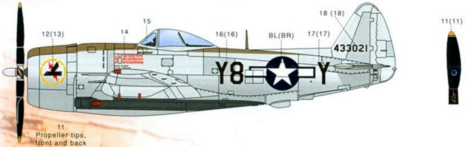
Aircraft 2 - P-47D-30-RA, flown by Lt. William Lee, 507FS, 404FG. This aircraft wears the 1st version of the Thunderbird logo designed by Lt. Lee. It became the group's unofficial insignia near war's end. Aircraft was later named "Tin Hornet". Overall natural metal finish with OD antiglare panel. Note Black belly paint to hide exhaust stains. Red bomb racks sway braces.
